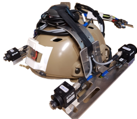
Fig. 2. The helmet used for the acquisitions. The IMU SBG-Ellipse-N sensor that includes the magnetometer, the IMU and the GNSS is on top of the helmet while the four cameras FLIR Blackfly S are on the sides.
