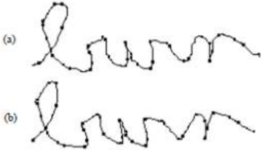
Fig. 4: (a) Control points extracted from the original strait. (b) Reconstructed strait using control points and B-splines
