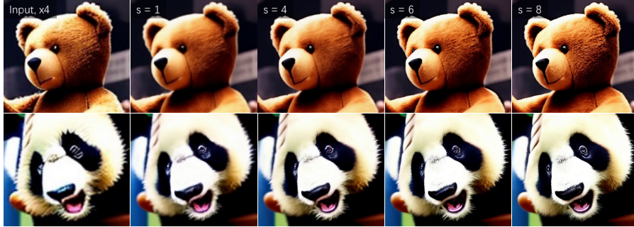
Figure 5: The effectiveness of video-aware conditioning. For video super-resolution ( 4\times ), we modify the input downscaling factor from s = 1 to s = 8 , and more texture details are generated. Zoom in for best view.
