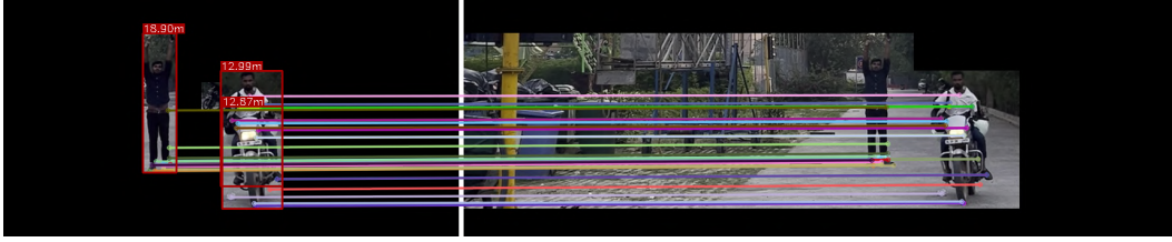
Figure 7: Illustration of masked keypoint detection and matching in left and right frames (separated by the white border). The left frame shows the detected objects and the estimated depths. Keypoints are concentrated within the object bounding boxes in the left frame and their expanded parallax regions in the right frame, demonstrating reduced processing area.
