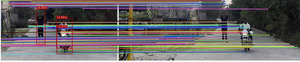
Figure 6: Illustration of unmasked keypoint detection and matching in left and right frames (separated by the white border). The left frame shows the detected objects and the estimated depths. Note the distribution of keypoints across both relevant objects and irrelevant background areas.
