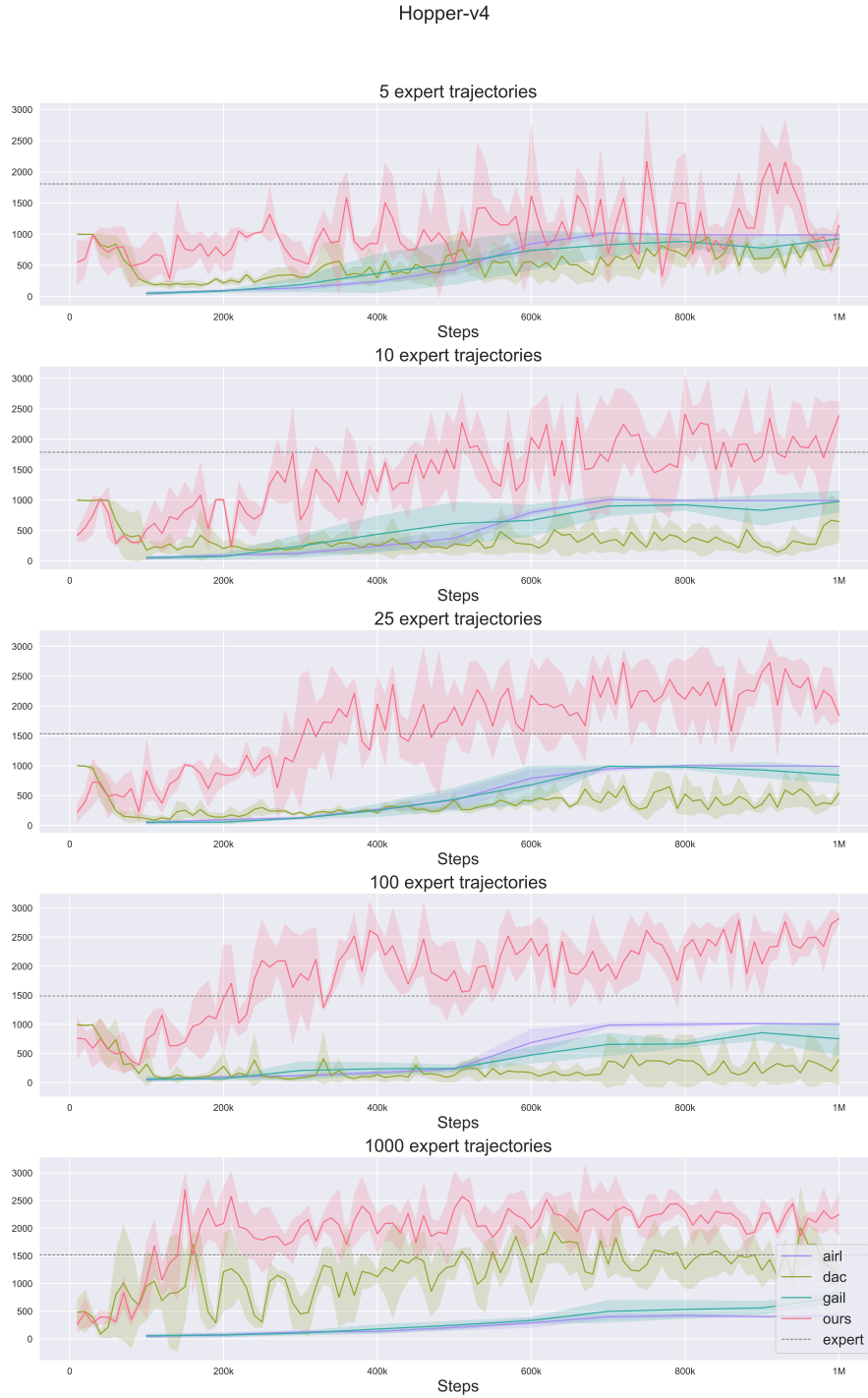
Figure 5: Training return diagram averaging across three seeds for different numbers of expert trajectories in Stochastic Hopper-v4.
