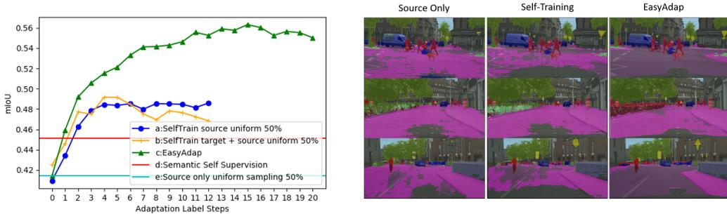
Figure 2: Left: Best mIoU per adaptation step; self-training (a); self-training+uniform sampling on target domain (b); self-training+uniform sampling+semantic self-supervision (c); uniform sampling+semantic self-supervision (d); uniform sampling source only (e). Right: Qualitative examples
