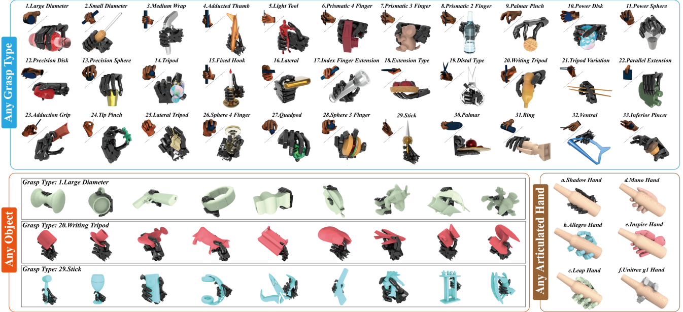
Fig. 1: For any grasp type in GRASP taxonomy [1], any object , and any articulated hand , our pipeline efficiently synthesizes contact-rich, penetration-free, and physically plausible dexterous grasps, starting from only one human-annotated grasp template to specify an initial hand pose and contact information per hand and grasp type.
