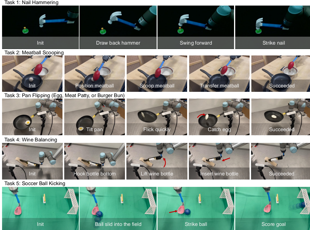
Figure 9: Policy Rollouts. We evaluate diverse real-world tasks: nail hammering (precision in locating a nail tip), meatball scooping (slippery object, constrained environments), pan flipping (extremely dynamic, high-speed, contact-rich), wine balancing (precise control of unstable objects), and soccer ball kicking (dynamic object handling, goal-directed actions).
