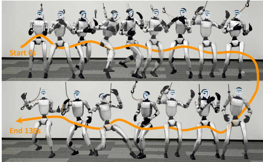
Figure 1: A general whole-body control policy in the real world tracks the motion of two consecutive long-duration actions, with a total duration of approximately 135 seconds. A boxing sequence appears at the top of the image, with a Charleston dance shown at the bottom.
