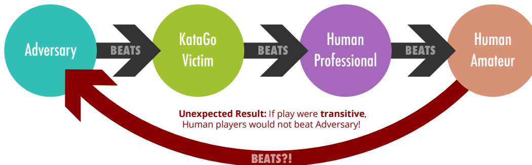
Figure 2: A human amateur beats our adversarial policy (Appendix F.1) that beats KataGo. This non-transitivity shows the adversary is not a generally capable policy, and is just exploiting KataGo.
