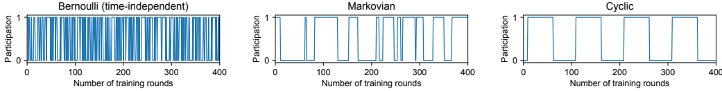
Figure C.6.1: Illustration of different participation patterns, in the first 400 rounds of a single client with 52.7% mean participation rate.
