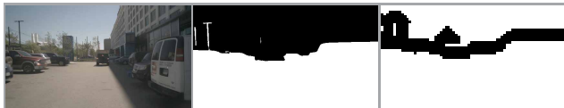
Figure 4. (Left) Real-world image. (Middle) Semantic segmentation of safety-critical regions. (Right) The buffer zone is introduced by dilating the safety-critical mask, shown in black. Loss is not computed in the buffer zone.
