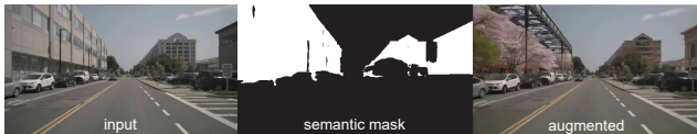
Figure 2. Given an input image sequence, we compute inpainting regions using semantic segmentation. The resulting masks guide VACE’s inpainting process to augment static scene elements into a Tokyo-style appearance.
