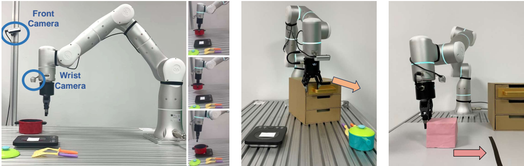
Figure 8: Real world setting. 1. Pick-and-Place : use the gripper to pick the red pot up and place it onto the black induction cooker. 2. Articulated-Manipulation : use the gripper to open the drawer. 3. Push-cube : use the gripper to push the cube across the black line.
