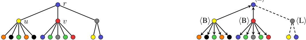
Figure 3: ROOTNEIGHBORS examples. Left: Example tree for ROOTNEIGHBORS. Right: Example of an optimal directed subgraph over the input tree, where the nodes with a degree of 6 ( u and v ) BROADCAST, while other nodes LISTEN.
