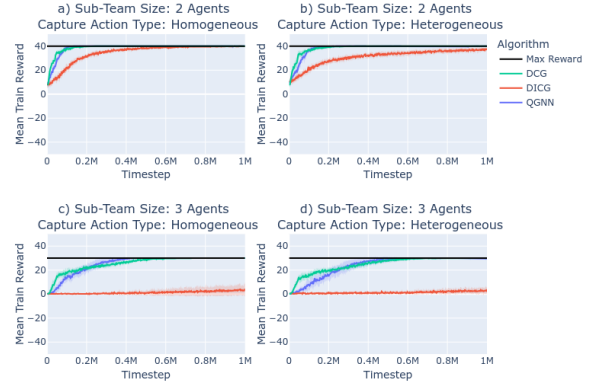
Figure 5: Train episode reward (Mean and shaded Standard Deviation) for ten independently trained models. The miscapture penalty was disabled for these training iterations. The Full CG topology was used, except for DICG which used an Attention mechanism to create the graph. Note with the miscapture penalty disabled the task no longer satisfies the requirements for an MST and was solved by all SOTA methods.
