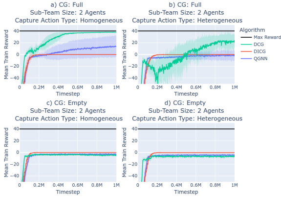
Figure 4: Train episode reward (Mean and shaded Standard Deviation) for ten independently trained models. The Full CG topology was used for (a) and (b), except for DICG which used an Attention mechanism to create the graph. For (c) and (d), the Empty CG topology was used for all algorithms. Note that communication is necessary for MSTs but is not sufficient when complexity increases.
