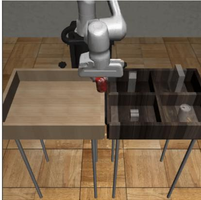
(b) Can Pick-and-Place Environment (Mandlekar et al., 2021). The grasper must pick up a can from the left bin and place it into the correct bin on the right side.
