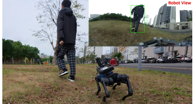
Fig. 1. A scenario of a quadruped robot following a person through a rugged lawn. The robot view is from an onboard panoramic camera (see Sec. IV-C). The robot’s dynamic motion induces severe camera ego-motion and vibration, which bring challenges for person localization.
