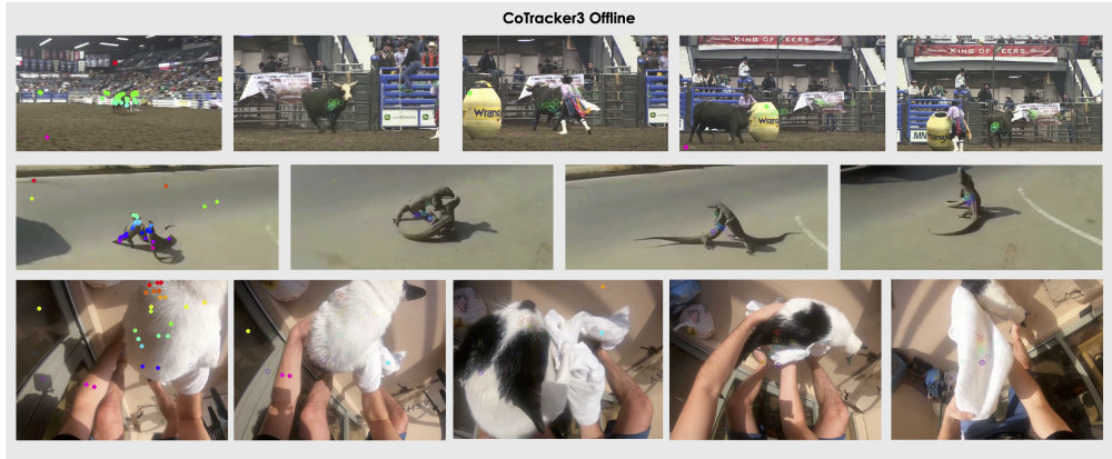
Figure 7: Challenging ITTO videos for CoTracker3 offline. Visualization of the three videos with the lowest Average Jaccard (AJ) scores for CoTracker3 offline. Offline model struggles on the same three videos as the online variant, however tracks remain on the bull in the third visualized frame, and drift off the bull in the fourth frame, before being placed back on the bull again in the last frame, the inverse of the online version. All tracks are incorrectly predicted as occluded in these frames.
