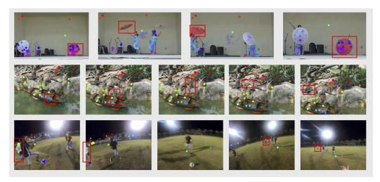
Figure 2: **CoTracker3 on ITTO.** Points tracked by color & red boxes added for illustration. Top: model biases red umbrella tracks to the right panel and fails when the girls switch positions. Middle: model struggles to track individual monkeys, which have repeated features. Bottom: model fails under camera-to-object distance changes. Background points are tracked with near-perfect accuracy.
