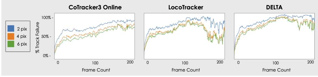
Figure 3: Catastrophic Track Failure. Track failure rates over time for 2, 4, and 6 pixel thresholds. CoTracker3 and DELTA suffer rapid and irrecoverable degradation once tracks leave their native resolution window. LocoTrack is more resilient, likely due to its global track initialization stage.
