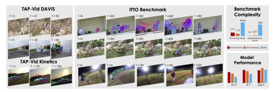
Figure 1: **Overview of ITTO benchmark vs. other benchmarks**. ITTO has more objects per video, highly deformable objects (such as umbrella opening and closing in top row) and all phenomena of the real world (significant % of moving tracks, and high track reappearance count). SOTA tracking methods perform worse on ITTO compared to the existing benchmark; e.g. CoTracker3 [17] performance drops from 61.8 to 35.5 for Average Jaccard (AJ) and from 76.1 to 47.1 for  $\delta$ .
