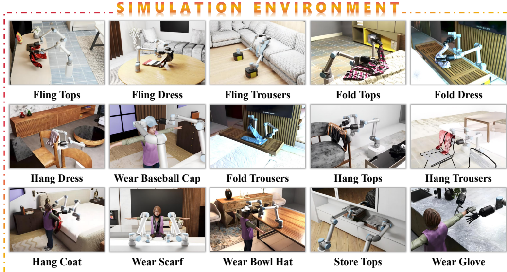
Figure 4: DexGarmentLab Simulation Environment. We introduce 15 garment manipulation tasks across 8 categories, encompassing both garment-self-interaction (e.g., Fling, Fold) and garment-environment-interaction (e.g., Hang, Wear, Store) scenarios. In garment-self-interaction tasks, key variables include garment position, orientation, and shape. In garment-environment-interaction tasks, environment-interaction assets positions (e.g., hangers, pothooks, humans, etc.) are also considered.
