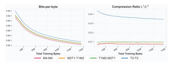
Figure 8: Encoder-decoder architecture ablation using raw byte inputs. Validation BPB (left) and compression ratio  $L^1/L^0$  (right) for H-Net (1-stage) throughout training. We evaluate four encoder-decoder ( $\mathcal{E}^0-\mathcal{D}^0$ ) configurations: M4-M4 , M2T1-T1M2 and T1M2-M2T1, and T2-T2, where M denotes Mamba layers and T denotes Transformer layers.
