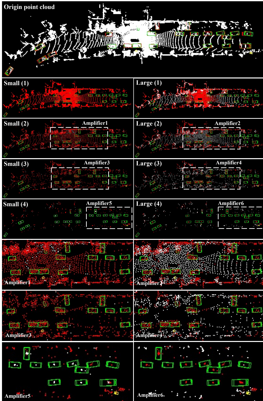
Figure 5: Visualization results on Waymo val set. The red and green 3D boxes in figures are ground truth and prediction boxes. Green, cyan, and yellow represent Car , Pedestrian , and Cyclist . Red and white points represent activation and blocking points, respectively. "Small" and "Large" means the scale of group in MSG, and the digital in parentheses is the index of SA layer.
