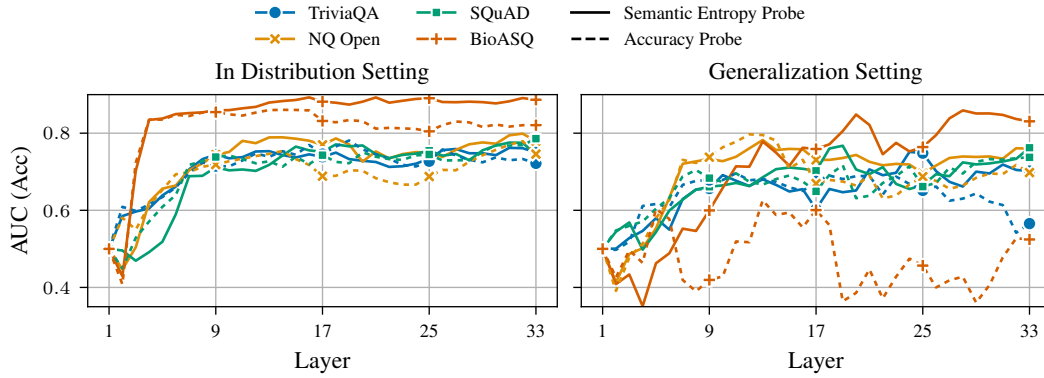
Figure C.8: SEPs predict model hallucinations better than accuracy probes when generalizing to unseen tasks (right). In-distribution, accuracy probes have comparable performance (left). Mistral-7B in the short generations setting with probes trained hidden states from the SLT. For the generalization setting, probes are trained on all tasks except the one that we evaluate on.
