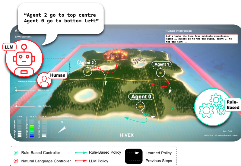
Figure 1: The Aerial Wildfire Suppression environment includes two types of controllers: Natural Language-based and Rule-Based. Controller interventions are passed to the LLM-Mediator, temporarily providing actions and overwriting the agents’ learned policy actions.
