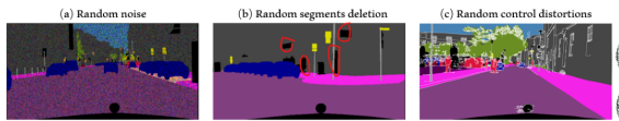
Figure 5: Data augmentation techniques on control images: (a) adding random Gaussian noise, (b) deleting random segments from the image for more generation robustness, (c) distorting the control images.
