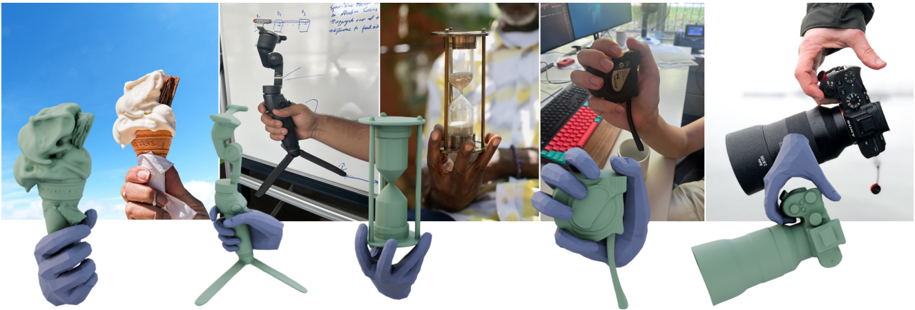
Figure 1. In-the-wild results. From a single RGB frame from in-the-wild (top row), our method reconstructs detailed 3D hand-object interactions (bottom row). It does so by guiding a latent diffusion model with multi-modal cues derived from the input image and several foundation models.
