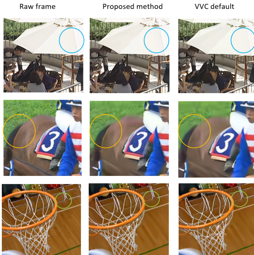
Figure 3. Visual comparison of raw frame, VVC default filtering and our split luma-chroma model. From top to bottom: BQTerrace, RaceHorses and BasketballDrill.
