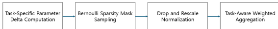
Figure 4: DARE-TIES Merge Kernel. The figure illustrates the DARE-TIES merge procedure applied after tensor alignment by the Architecture Mapper. Parameter deltas relative to a shared base model are sparsified via Bernoulli masking, rescaled to preserve expected magnitude, and combined using genome-specified mixing coefficients. The exact formulation of the merge kernel is provided in Appendix C.3.
