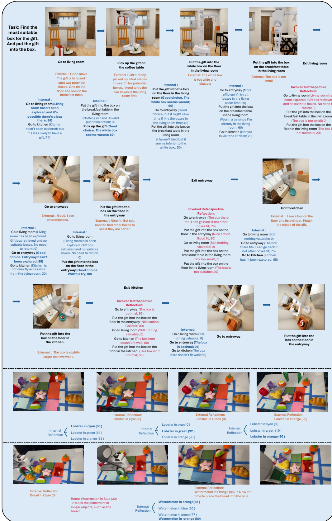
Figure 8. Steps and reflections are simplified for better presentations. Blue text shows internal reflection used for candidate selection, orange text shows external reflection after execution. We put reflection scores inside brackets. Red text shows retrospective reflection and model updates.
