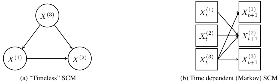
Figure 1: Structural Causal Models (SCMs) describing causal relationships. The inter-variable relationships are the same between the two SCMs, with the time-dependent SCM treating the dependency as occurring across a single time-step.
