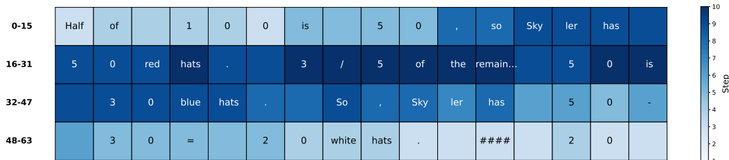
Figure 4: Visualization of Decoding Steps on GSM8K. Tokens are color-coded by their decoding step (lighter = earlier, darker = later). Thresholds are set to \tau_{\text{high}} = 0.9 , \tau_{\text{low}} = 0.4 , with remasking disabled. The figure illustrates that multiple tokens are generated in a single step, while each sub-decoding area reliably commits at least one token, consistent with the intended hierarchical decoding behavior.
