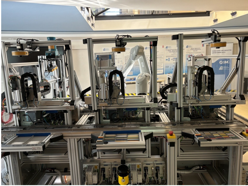
Figure 1: Complete pen production line showing integrated robotic stations
