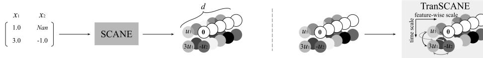
Figure 2: Concept of SCANE and TranSCANE: The leftmost matrix is an input time series data with m = n = 2 . x_1 and x_2 represent two variables. Nan means missing. \mathbf{u}_1 and \mathbf{u}_2 are the feature embedding \in \mathbb{R}^d of the feature x_1 and x_2 , respectively. After SCANE, all observations will be mapped based on their feature embeddings proportional to the observed values, while missing values will be mapped to \mathbf{0} = \mathbf{0}^d . The right figure shows the interaction of SCANEs in the transformer encoder. TranSCANE facilitates the variable interacting flexibility across time scale and feature-wise scale.
