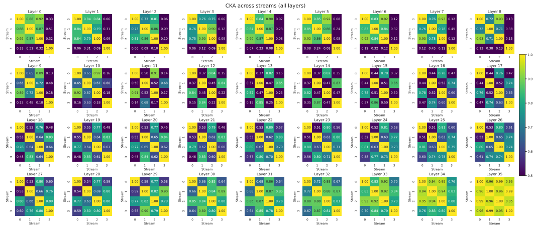
Figure 4: Within-layer CKA similarity matrices across depth. Middle layers show clear block structure, reflecting soft partitioning into redundant stream subgroups.
