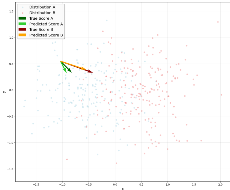
Figure 10: Computing relative Fisher information. Our model predicts \nabla \log g(x_i) at query points x_i via cross-attention with the samples y_i \sim g . These predicted scores can be used to estimate the relative Fisher information.
