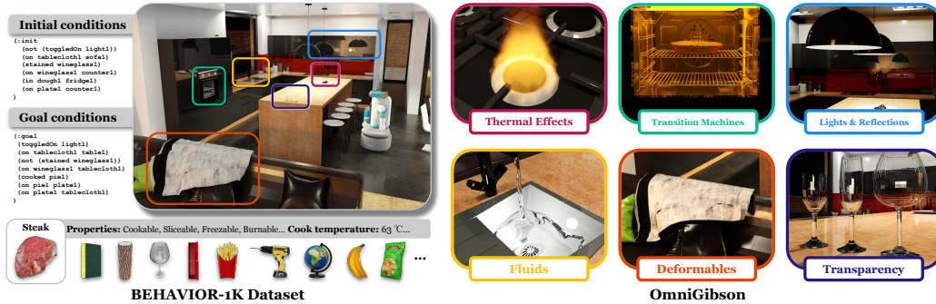
Figure 2: Elements of BEHAVIOR-1K. Our benchmark comprises two elements: BEHAVIOR-1K DATASET and OMNIGIBSON. Left: BEHAVIOR-1K DATASET includes 1,000 BDDL activity definitions (top left), 50 realistic and diverse scenes (top right), and 5,000+ objects with properties annotated in the knowledge base (bottom). Right: OMNIGIBSON provides the necessary functionalities to realistically simulate the 1000 activities, including thermal effects such as fire/steam/smoke (top left), fluid dynamics (bottom left), functional machines for transition rules (top center), deformable bodies/cloths (bottom center), realistic lighting and reflections (top right), and transparency rendering (bottom right). Together, they constitute a concrete, realistic instantiation of an everyday activity like CookingDinner in simulation.
