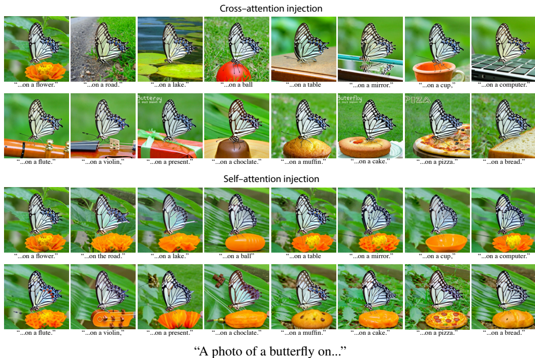
Figure 16: Object preservation and replacement using cross and self attention injection. Top: by injecting only the cross-attention weights of the word “butterfly” taken from the top-left image we can preserve the structure and appearance of a single item while replacing its context (i.e., background). Bottom: using only self-attention injection we can’t specify which object should be preserved, therefore, modifying the background while keeping the butterfly is more challenging.
