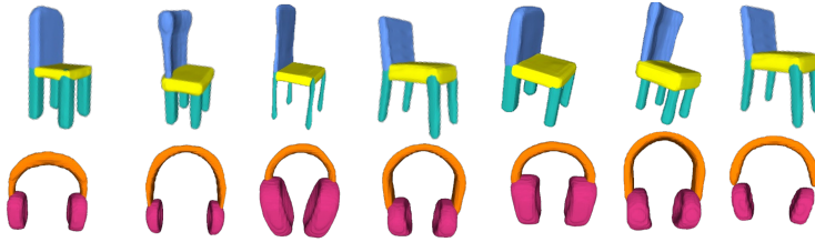
Figure 7: Visual results on ShapeNet when fitting multiple primitives to the target shapes. The number of primitives used is given as prior. We employ 3 and 2 primitives for chairs and earphones, respectively. Semantic consistency within the same category is illustrated with colors.
