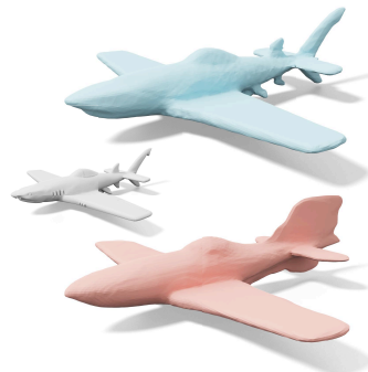
Figure 3: Latent-encoded SDFs (red) struggle to reconstruct “unique” features (grey, plane’s tail) despite training on a single class of objects (planes). Our representation (blue) does not. gpvillamil under CC BY.
