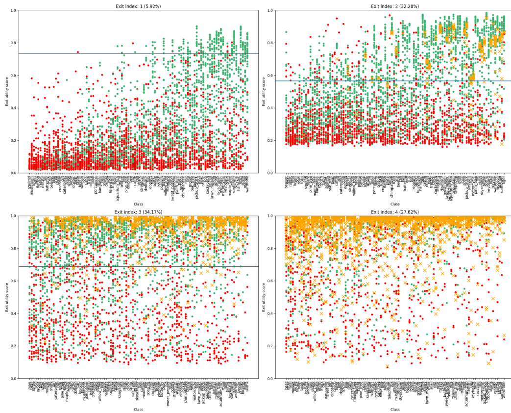
Figure 9: Distribution of samples to different exits under the average latency budget of 8 milliseconds.
