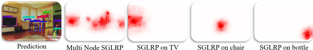
Figure 5: Difference between relevance maps from SGLRP and Multi-Node SGLRP. The relevance maps are for YOLOv3 (Redmon & Farhadi (2018)).
