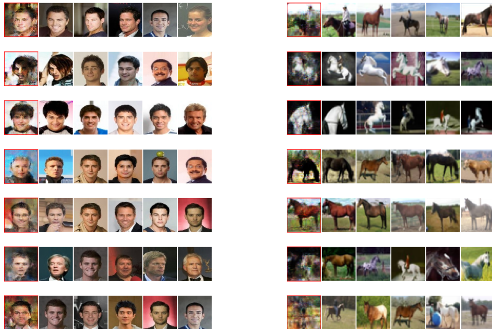
Figure 17: Comparison between the images generated by WGAN-GP trained on 256 images and the nearest neighbors (measured by SSIM) from the training set. Images with red bounding boxes are generated images.
