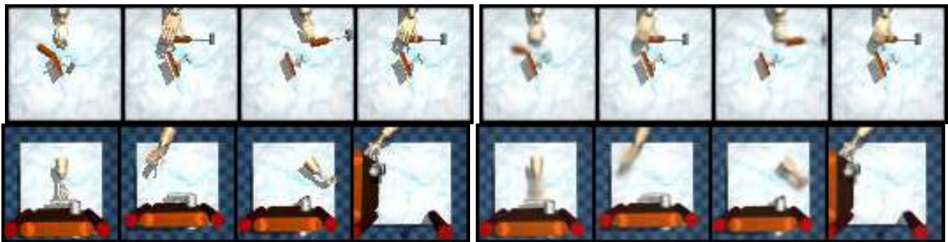
Fig. 11. ROW1: Original input images of the Hammer task; ROW2: Corresponding Reconstructed images; ROW3: Original input images of the Door task; ROW4: Corresponding Reconstructed images. These images depict that the latent features sufficiently encodes features required to reconstruct the images.
