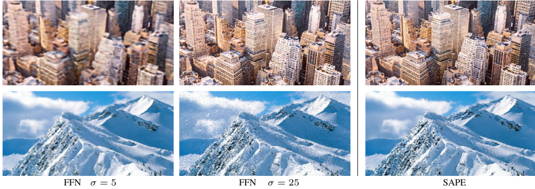
Figure 1: Left: Fourier Features Network (FFN) encoding, tuned to a bandwidth of low frequencies in order to fit the smooth regression. The same frequency bandwidth yields blurry buildings in the top image. Middle: FFN tuned to a higher bandwidth to fit the sharp details of the city. The same bandwidth results in the appearance of noisy artifacts in the mountain image. Right: SAPE is able to fit both examples without extra tuning, using the same choice of frequency bandwidth in both cases.
