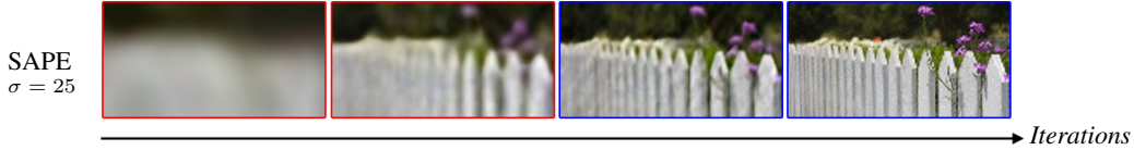
Figure 4: Learning progress of SAPE for implicit representation of a 2D image, showing iterations 75, 150, 300 and 3000 (left to right). The beginning of optimization is dominated by low frequencies: spectral bias maintains global optimization stability. As the optimization progresses high frequency mapping takes place, and SAPE fits the finer details of the image. See other methods in the appendix.
