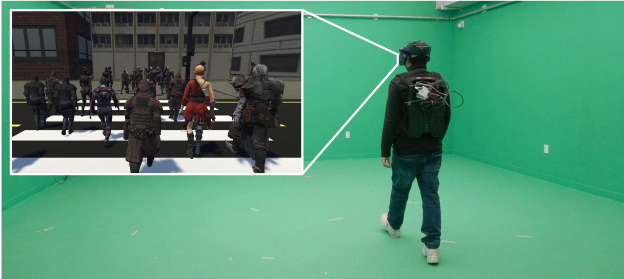
Figure 1: A participant walking in the motion capture studio and moving toward the opposite sidewalk in the virtual metropolitan city, and a third-person view of the virtual environment and virtual crowd the participant was observing. The participant is wearing all of the devices used in this study (an MSI VR One backpack computer, and an HTC Vive head-mounted display).
