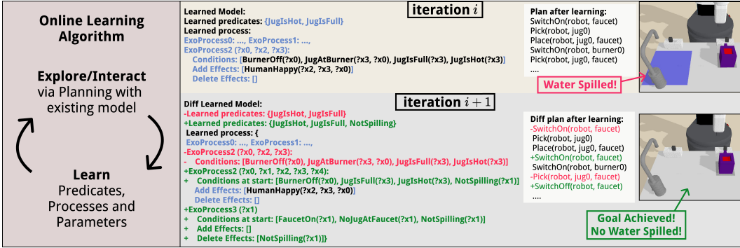
Figure 3: The online learning loop, where the agent repeatedly uses its current model to plan and interact with the world, then refines that model by learning new predicates and causal processes from the experience. The figure shows an example where the agent’s initial model in iteration i leads to a failed plan (Water Spilled!). After observing this failure and updating its knowledge (“Diff Learned Model”), the agent creates a successful plan in iteration i + 1 (“Diff plan after learning”).
