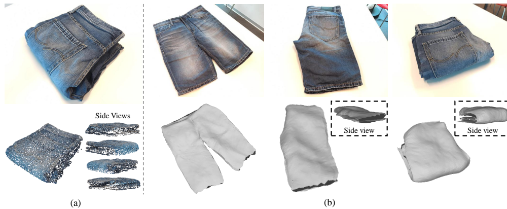
Figure 7: Real-world evaluation. (a) The captured image and point cloud of the pants. (b) Our reconstructed results.
