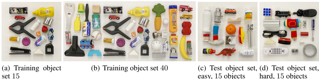
Figure 8: The train/test object sets. Objects need to be graspable of the gripper at any configuration (smaller than the gripper open width and has enough height), and need to be able been captured by the depth camera (no transparent nor has thing wall).
