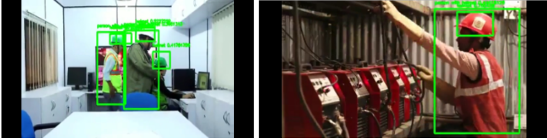
Figure 2: (Detection of persons wearing and not wearing helmets different work environments.
