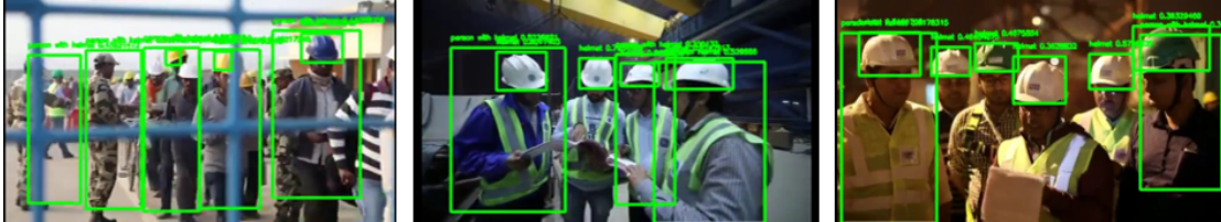
Figure 1: (Detection of persons wearing and not wearing helmets in a large group in factory settings.
