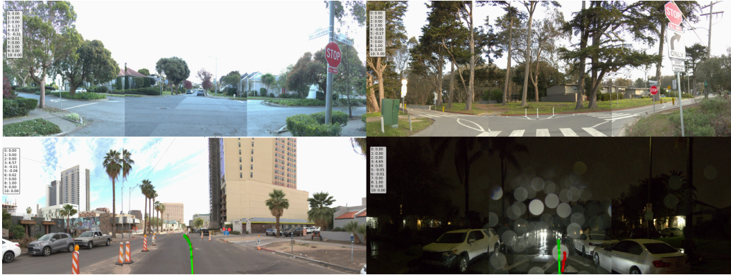
Figure 8: Qualitative Results on the WOD Vision-Based E2E Driving Dataset. The red trajectory shows the predictions of RAP-DINO, and the green trajectory denotes the ground-truth future path. Across the four examples, RAP-DINO successfully identifies a stop sign, traffic cones, and oncoming vehicles at night, leading to accurate and safe trajectory plans.
