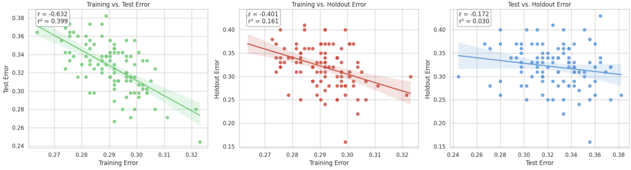
Figure 2. Synthetic data generated from 10 variables then taking a weighted linear combination of 3 variables making them determine the target label for each instance. Then randomly flipping the bits of 30% of the data, the data contained 1,000 instances. We then performed 100-fold cross validation AdaBoost, with 50 base learners. There were a thousand instances generated and 10 features for this data set. The data was partitioned into train, test, and hold-out as follows: initially 10% was reserved as the hold-out set, then 67.5% of the data was devoted to the training set and the remaining 22.5% to the test set.
